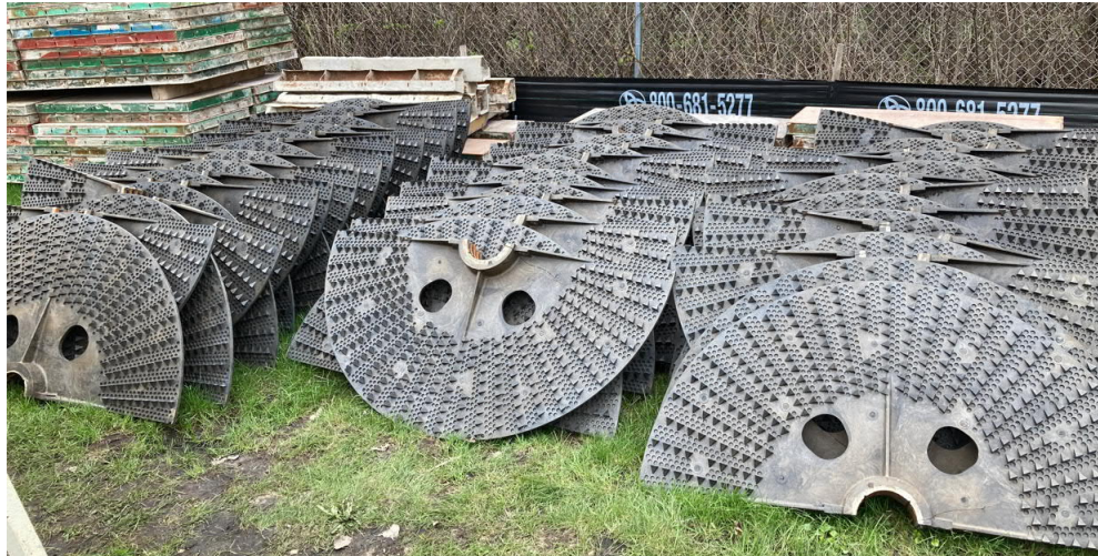
Photo 1: Existing discs with cracks when removed from service
